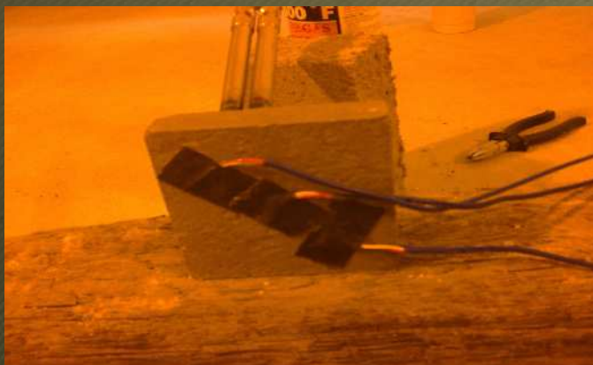
Figure 2: Distribution of Thermocouple on Non-Exposed Surface
