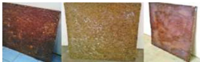
Fig. 5: Panel board from binder polyester resin + hardening catalyst
